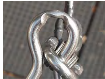
Swing yoke worn 2/3 through, Priority One Immediate Attention
