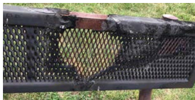
⑤ FIRE DAMAGED BENCH
