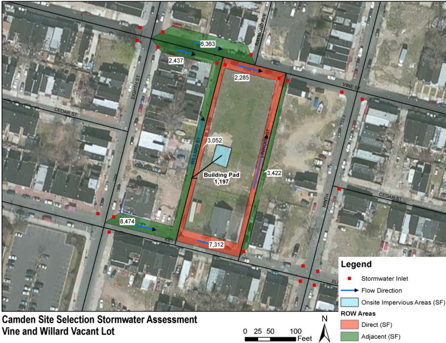
FIGURE 4-7: VINE AND WILLARD VACANT LOTS - STORMWATER ASSESSMENT
