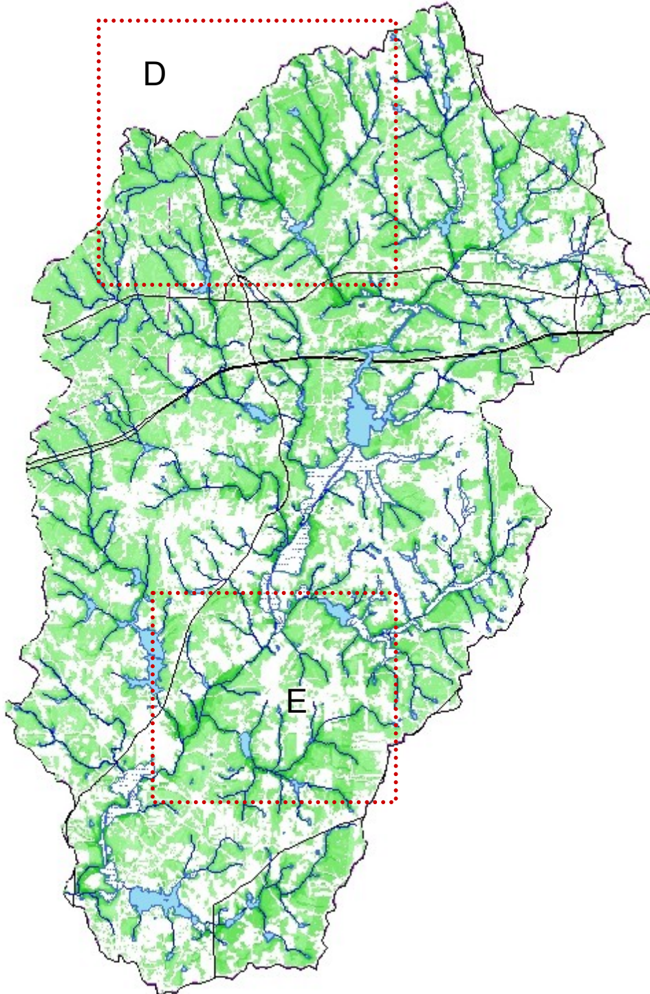
Figure 3 – Conservation Priority Index (CPI) for forests and wetlands in the upper Little Tallapoosa River watershed, Georgia. The darkest hues have the greatest potential importance for source water pollution prevention or mitigation. Enlarged areas (D and E) are shown in Figure 5.
